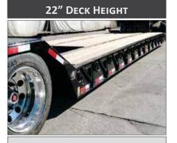
With a standard deck height of 22", Globe Trailers have lower overall height, which allows taller loads to be hauled.
