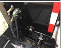
Air, electric and hydraulic (when applicable) fittings are all centrally located at the base of the gooseneck inside a bolster. This makes for quick and easy connect and disconnect. The fittings are protected from possible contact with equipment being loaded or unloaded.
