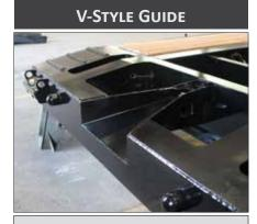
V-Style guide with front tapered beams helps position the gooseneck locking pin, which makes hooking up to a Globe Trailer fast and easy. The locking pin guide rim helps prevent the gooseneck locking pin from coming loose in transit.
