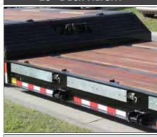
With a standard deck height of 18", Globe Trailers have lower overall height, which allows taller loads to be hauled.
