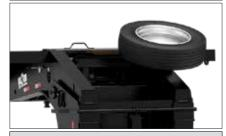
Optional spare tire that mounts securely on top of Gooseneck.
