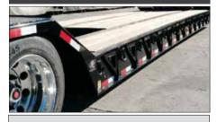
With a standard deck height of 18", Globe Trailers have lower overall height, which allows taller loads to be hauled.
