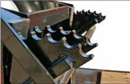
Multi Position Ride Height options. Makes adjustments for various 5th wheel heights easy and allows for larger ground clearance or lower deck height.
