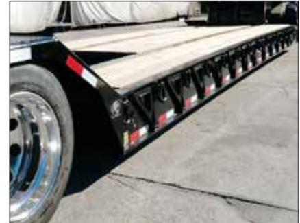
With a standard deck height of 18", Globe Trailers have lower overall height, which allows taller loads to be hauled.
