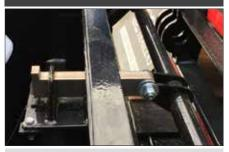
Globe Trailers air lock with safety bar and spring extended pin ensures that the gooseneck locking pin will remain secured even if air pressure is lost.
