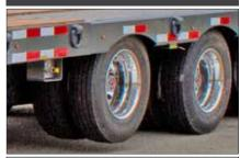
Lift Axle distributes the load carrying capacity on the other axles, also increases the tire & axle life over wear & tear. Keep lifted in unloaded, and grounded in loaded conditions.
