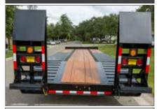
Adjustable with spring assist and safety bar.
