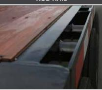
2 ½" rolled formed steel. 6" Structural Channel @ 6.5 lbs/ft, 5/16" Thick Stake Pockets 1 5/8" x 3 ½" x ¼", 24" O/C, ¼" x 3" Rub rail.
