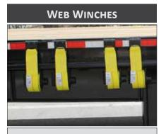
Web winches are welded on, located on the road side. Used to retain loads and objects on the trailer.
