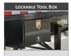
Optional Lockable Tool Box Mounted Underside of Main Deck, 24" x 24" x 48" Steel, can be located on either side.
