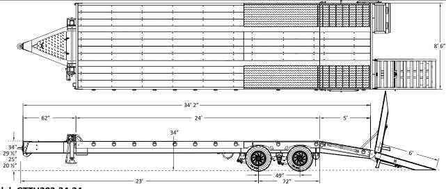
Trailer Model: GTTU202-34-24 Weight: Apx. : \_\_\_\_\_ ± lbs
