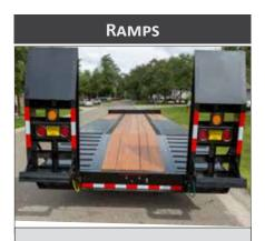
Adjustable with air powered and safety bar.
