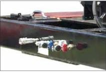
The front side of the neck offers easy access for connections like hydraulics, electrical and air lines.
