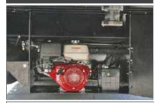
Gasoline 27 HP Pony Motor provides hydraulic operation when disconnected from the trucks wet line. Unit is self contained under the neck.
