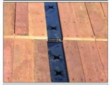
Double slotted key holes gives you more tie-down angles for securing load.
