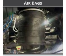
30,000 pound rated large diameter air bags are standard. This allows for lower operating pressure and higher capacity when needed.
