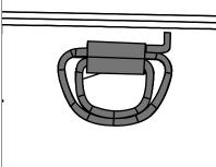
"D" ring tie downs on upper and lower deck with a design load of 15,000 lbs.
