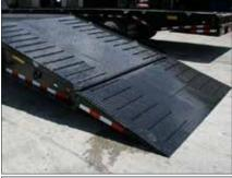
The Hydraulic Tail is a bi-fold that extends to allow easy loading of equipment with a very low load angle. In the transportation mode the flip under ramp folds into the beaver tail for a shorter overall trailer length.
