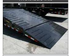
The Hydraulic Tail is a bi-fold that extends to allow easy loading of equipment with a very low load angle. In the transportation mode the flip under ramp folds into the beaver tail for a shorter overall trailer length.
