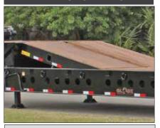
The Hydraulic Ramps extend to allow easier loading on to the upper deck.
