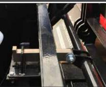
Globe Trailers air lock with safety bar and spring extended pin ensures that the gooseneck locking pin will remain secured even if air pressure is lost.
