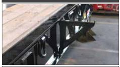
Standard heavy duty outriggers that span the entire height of the side rail allow for maximum force to be applied when in use.
