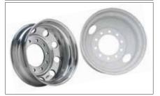
All Globe trailers come with standard HUB piloted disc wheels. Wheels are also available in all Aluminum or Outer Aluminum.
