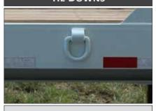
D-rings on each side of the deck make it easier to secure loads to the trailer.
