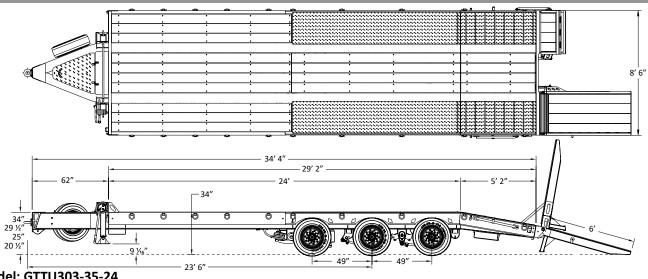
Trailer Model: GTTU303-35-24 Weight: Apx. : \_\_\_\_\_ ± lbs
