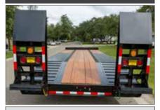
Air adjustable ramps and safety bar.
