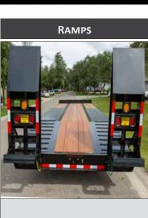
Adjustable with spring assist and safety bar.
