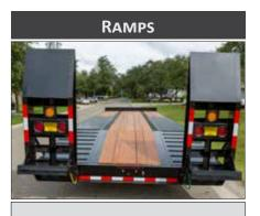
Adjustable with spring assist and safety bar.
