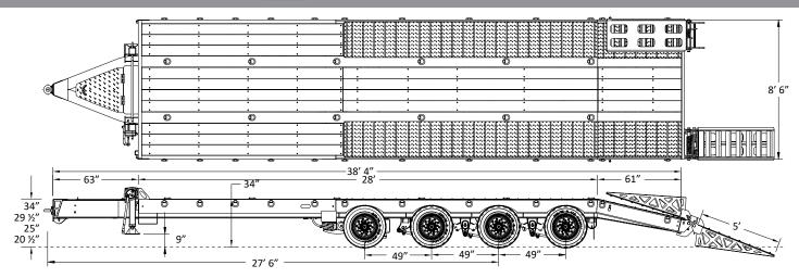
Trailer Model: GTTU304-38-28 Weight: Apx. : \_\_\_\_ ± lbs
