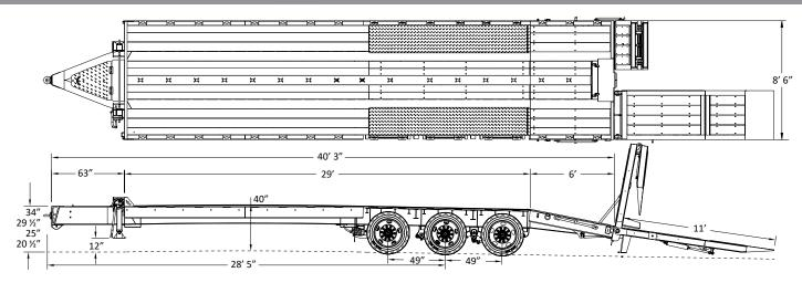
Trailer Model: GTTU303-40-28 Weight: Apx. : \_\_\_\_ ± lbs
