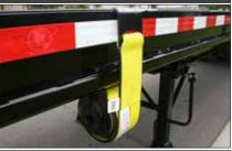
Web winches can be located on either side. Used to secure loads and objects on the trailer.
