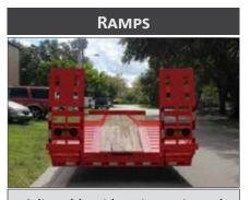
Adjustable with spring assist and safety bar.
