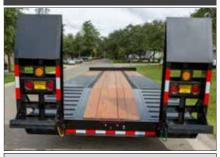
Adjustable with spring assist and safety bar.
