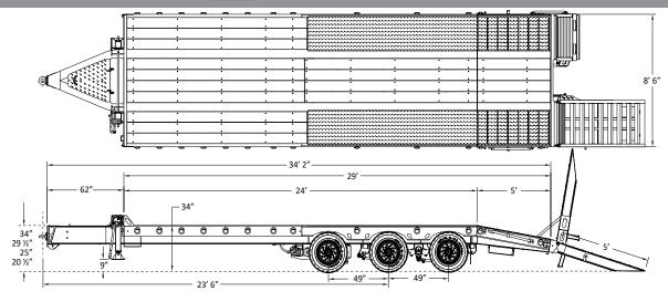
Trailer Model: GTTU253-37-24 Weight: Apx. : \_\_\_\_ ± lbs
