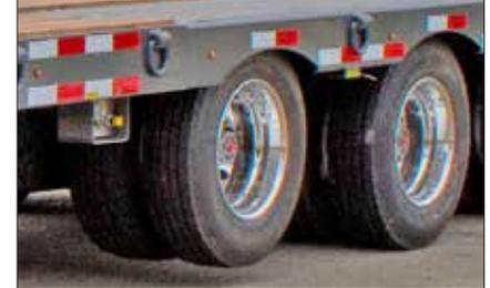
Lift Axle distributes the load carrying capacity on the other axles, also increases the tire & axle life over wear & tear. Keep lifted in unloaded, and grounded in loaded conditions.
