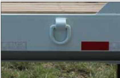
D-rings on each side of the deck make it easier to secure loads to the trailer.
