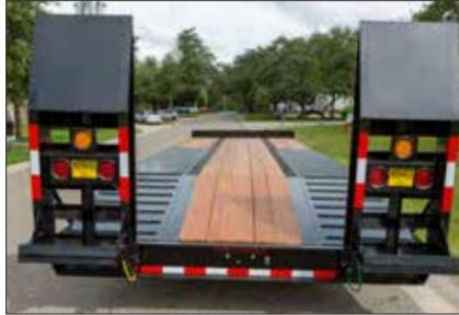
Adjustable with spring assist and safety bar.
