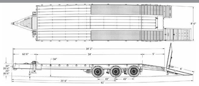
Trailer Model: GTTU253-35-24 Weight: Apx. : \_\_\_\_ ± lbs
