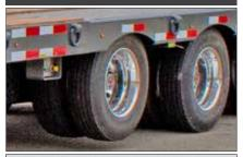
Lift Axle distributes the load carrying capacity on the other axles, also increases the tire & axle life over wear & tear. Keep lifted in unloaded, and grounded in loaded conditions.
