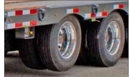
Lift Axle distributes the load carrying capacity on the other axles, also increases the tire & axle life over wear & tear. Keep lifted in unloaded, and grounded in loaded conditions.
