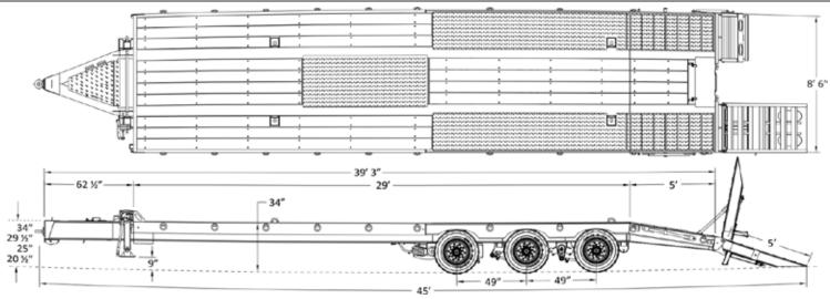
Trailer Model: GTTU253-39-29 Weight: Apx. : \_\_\_\_ ± lbs
