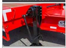
2 speed Landing Gear, allows for 160,000 lbs static load.
