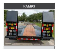
Adjustable with spring assist and safety bar.
