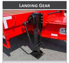
2 speed Landing Gear, allows for 160,000 lbs static load.
