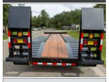
Adjustable with spring assist and safety bar.
