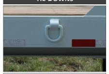
D-rings on each side of the deck make it easier to secure loads to the trailer.
