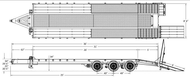
Trailer Model: GTTU253-37-26 Weight: Apx.: \_\_\_\_ ± lbs
