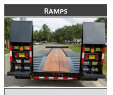
Adjustable with spring assist and safety bar.
