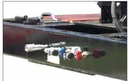
The front side of the neck offers easy access for connections like hydraulics, electrical and air lines.
