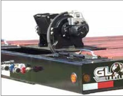
Available options for 10-45K lb hydraulic winch system. Mounted front and center of the upper deck. Standard cable length of 85' with shackle. Cable length options are available.
