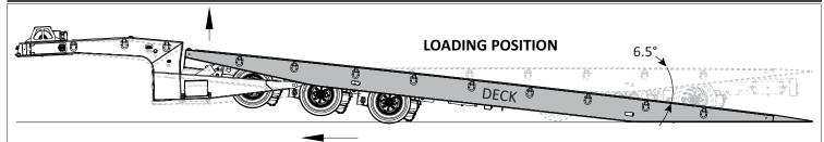
The axles travel forward and allow the deck to rise and allow for a very low 6.5 degree load position.
