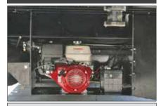
Gasoline 25 HP Pony Motor provides hydraulic operation when disconnected from the trucks wet line. Unit is self contained under the neck.
