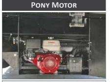
Gasoline 27 HP Pony Motor provides hydraulic operation when disconnected from the trucks wet line. Unit is self contained under the neck.
