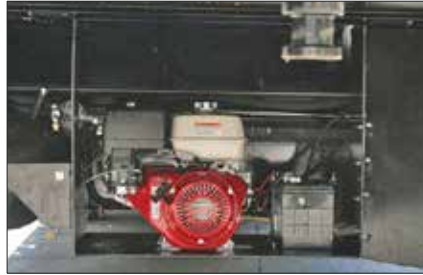
Gasoline 25 HP Pony Motor provides hydraulic operation when disconnected from the trucks wet line. Unit is self contained under the neck.
