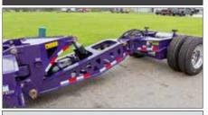
The Stinger Assembly increases the wheel base of the trailer when attached to the rear trailer frame. The Stinger Assembly is used for heavy hauling situations where regulations and specific axle loads must be adhered.
