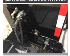
Air, electric and hydraulic (when applicable) fittings are all centrally located at the base of the gooseneck inside a bolster. This makes for quick and easy connect and disconnect.
