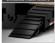
Standard Steel Front ramps, for ease of front loading.
