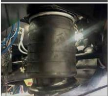
30K pound rated large diameter air bags are standard. This allows for lower operating pressure and higher capacity when needed.
