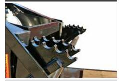
Multi Position Ride Height options. Makes adjustments for various 5th wheel heights easy and allows for larger ground clearance or lower deck height.
