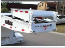
Flip box length options are available to achieve longer swing clearances when needed for longer truck frames or when coupling to single or multi-axle jeeps.
