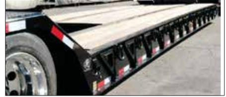
With a standard deck height of 18", Globe Trailers have lower overall height, which allows taller loads to be hauled.
