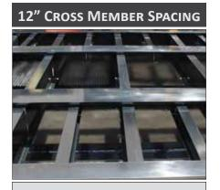
Standard 12" stubbed cross member spacing produces added strength to the trailer and also less stress on the decking, leading to a longer life of the decking material.
