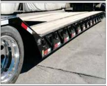
With a standard deck height of 18", Globe Trailers have lower overall height, which allows taller loads to be hauled.
