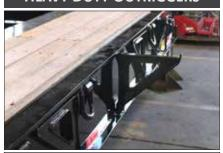
Standard heavy duty outriggers that span the entire height of the side rail allow for maximum force to be applied when in use.
