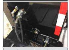
Air, electric and hydraulic (when applicable) fittings are all centrally located at the base of the gooseneck inside a bolster. This makes for quick and easy connect and disconnect. The fittings are protected from possible contact with equipment being loaded or unloaded.
