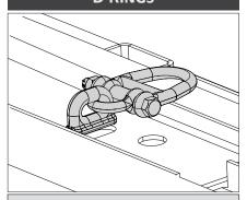
"D" ring tie downs on upper and lower deck with a design load of 15,000 lbs.
