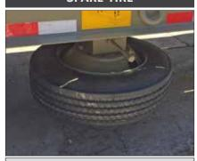
Spare tire and holder located on underside of trailer deck.
