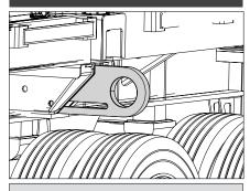
Two (2) lift rings on each side of deck for lifting aboard ships.
