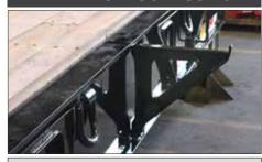
Standard heavy duty outriggers that span the entire height of the side rail allow for maximum force to be applied when in use.
