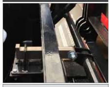
Globe Trailers air lock with safety bar and spring extended pin ensures that the gooseneck locking pin will remain secured even if air pressure is lost.
