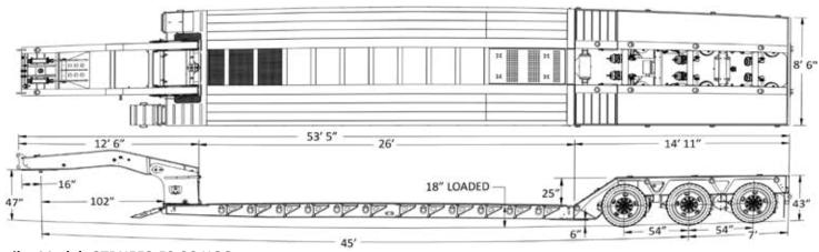
Trailer Model: GTBN553-53-26-HGG Weight: Apx. \_\_\_\_\_ ± lbs
