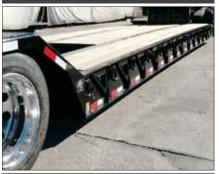
With a standard deck height of 22", Globe Trailers have lower overall height, which allows taller loads to be hauled.
